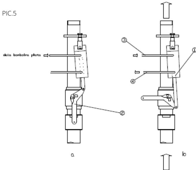
The gas is directed, by a flexible hose, from the nitrogen pilot cylinder to the piston in the inlet connection.
