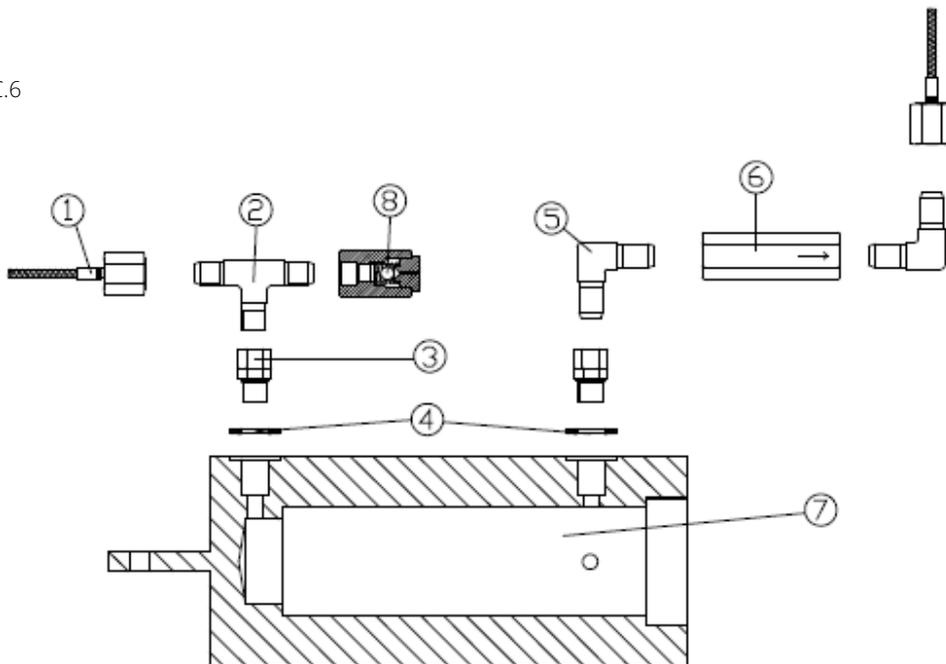
Components that can be installed on the directional valves: 1 flexible hose, 2 TEE, 3 nipple, 4 bonded seal, 5 elbow, 6 non return valve, 7 piston, 8 vent valve.
