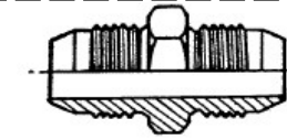
NIPPLIO JIC UNF-NF X JIC-UNF-NF CONO 74° NIPPLE JIC UNF-NF X JIC-UNF-NF 74° CONE
